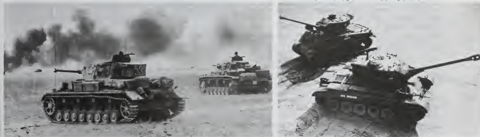
Figure 24: Tanks of World War II. (Left) German Pz. IV (foreground) and Pz. III (background) tanks, 1942. (Right) U.S. Army M26 Pershing tank with 90-millimetre gun (foreground) and M4 Sherman tank with 75-millimetre gun.
